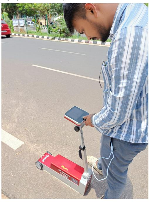
Enabled with 5.7" high-resolution color touchscreen, The retroreflectometer offers excellent visibility under all light conditions. The retroreflectometer logs all measurements with precise geolocation & provides comprehensive reports quickly with the help of user-friendly reporting software at ease.
